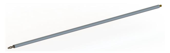
The measuring tip consists of a measuring stick with insulating bushel and a 4 mm bundle plug at the end. The measuring tip serves to measure the high voltage directly at the HV-electrode. It is screwed onto the measuring lance via a M4-thread. Instead of the measuring tip, a HV-cable with 4mm bundle- or banana plug may be plugged in directly
