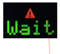
The zero point could be or cannot be maintained, e.g. error due to corona charge. The measurement result is not very useful.
