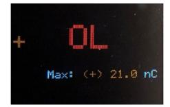
the measurement range for positive charges is exceeded (brown plus sign as prefix)
