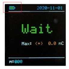
If the battery level display shows only one bar, the device should be charged with the supplied charger. If the battery level is too low, measurements are no longer possible.
