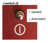
*Upward:* Turns on the device. Guides through the menu when turned on.
