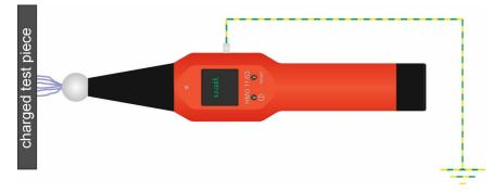
The ball electrode should be moved as perpendicularly as possible to the surface of the project; a grazing approach can lead to several, rapidly successive tuft discharges, whose individual charge pulses - if their interval is less than 10  $\mu$ s - would be added together. The result would then be an excessively high measured value.
