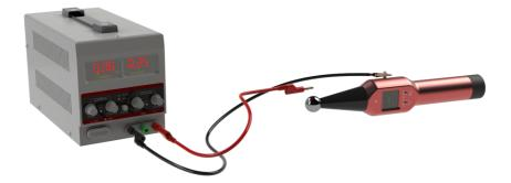
0.10 V at the laboratory power supply unit corresponds to 20 nC 0.25 V at the laboratory power supply unit corresponds to 50 nC 0.50 V at the laboratory power supply unit corresponds to 100 nC 0.75 V at the laboratory power supply unit corresponds to 150 nC
