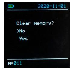
When turned on push the I-switch upward to get to the menu.
