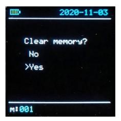
To delete the memory the query must be confirmed by pushing the R-switch down.
