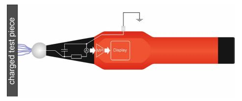
The charge transferred from the charged test piece via spark/brush discharge to the ball electrode is stored in capacitor C and then discharged to ground. The current, flowing across the measuring resistor, is measured. By an integral calculation, the charge is calculated from current over time.  $Q = I \cdot t$
