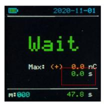
The second counter runs since releasing the "Reset switch" and stops when a measured value is recorded (this indicator can be switched off in the settings).
