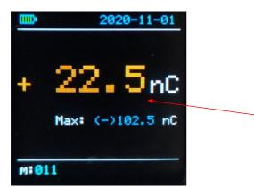
Display with measured value of positive polarity
