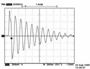
Discharge curve HV cable with polyolefin Conductor
