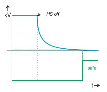
This means that the discharge process is fast at the beginning, however becomes proportionally slower. The smart-E 310 and smart-E 510 signal messages "safe" if the output voltage
