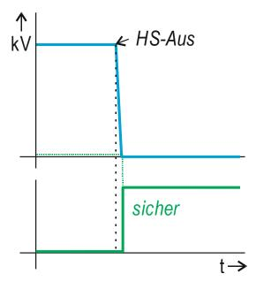
With a system capacity of 2 nF and an output voltage of 100 kV, the high-voltage is discharged within a second.
